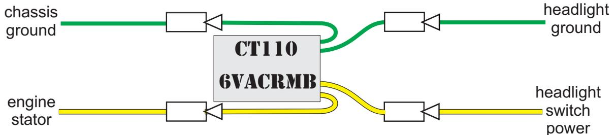
Connect Voltage Regulator (Yellow Male) to Engine Stator (Yellow Female)
